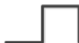
Figure 5 Waveform of encoded bit of bit of value 1 in the original serial data.
