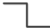
Figure 4 Waveform of encoded bit of bit of value 0 in the original serial data.
